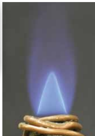
Stationary flame showing a defined flame front
