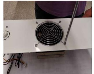
Turn over fan board and put it on heel blocks face up, remove screws and take out the fan cover
