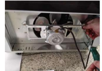
Take out motor wires from wiring hole on fan board, dismantle faulted motor and its holder from fan board, disconnect motor wires;
